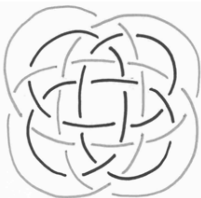
Fig. 11 - Spherical Covering Knot (second method) starting with a 4B x 3L Turk's head knot, similar to Ashley's knot #2232.
