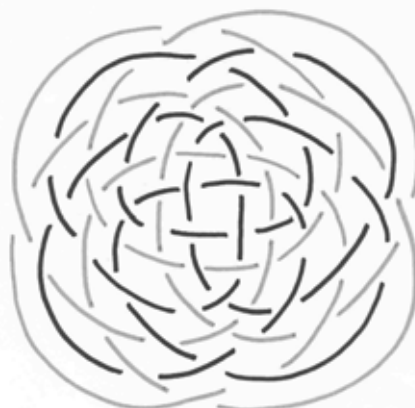
Fig. 12 -Spherical Covering Knot (second method) starting with a 4B x 5L Turk's head knot.
